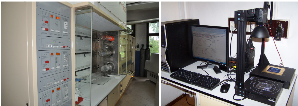
Fig. 3. The industrial quartz tube furnace for Si passivation in an ambient O_2 and diffusions processes using as a source the POCl_3 and BBr_3 (left) and WCT-120 photoconductance lifetime tester with optional Suns-Voc stage made by Sinton Consulting Inc. (right) in PV Laboratory of the IMMS.
