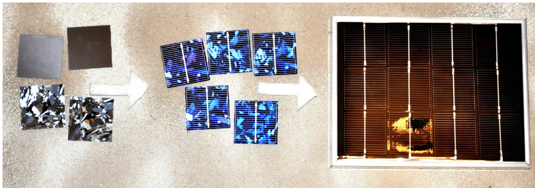
Fig. 2. Scheme of the basic stages on the way from silicon wafer to PV module under current investigation in Photovoltaic Laboratory of the IMMS.
