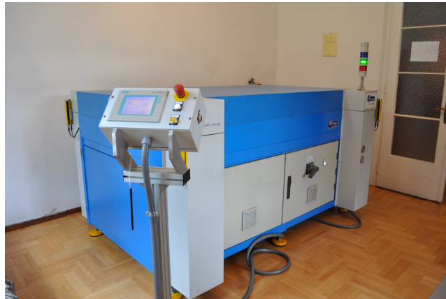
Fig. 4. The laminator in PV Laboratory allowing encapsulation of 1.5 m x 1.0 m modules.
