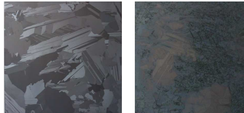
mc-Si before and after texturization process
