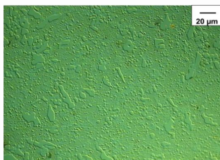
Fig 3 Microstructure of X210CrW12 steel after rolling – feedstock for thixoforming [15]
