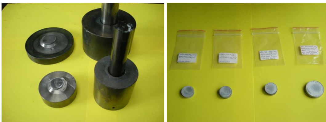
Fig.5 On the left heat resistant steel dies used for consolidation of powders at 600°C and pressure of 600 MPa On the right 20 and 30 mm discs consolidated at chamber shown in Fig.3 : 6061 + 20% ZrO 2 , 6061 + 20% Al 2 O 3 , Ax431 +10 % ZrO 2 i Ax431 + 10% ZrO 2 (30 mm).
