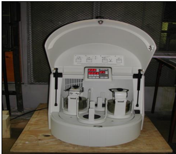
d. Fig.1 Planetary Frisch mill used for crushing of ribbons to obtain powders and above scheme of powder's refinement during
