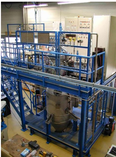
Fig. 2 Atomization facility at UTBM Belfort where metallic powder-atomizing in neutral atmosphere (argon) facility was erected in May 2003 at the original LERMPS facility where thermal spraying is performed.
