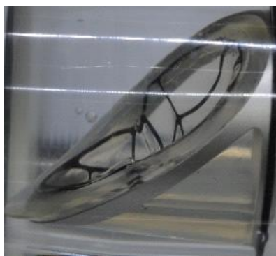
ZNP-Ti: flake deformation for: (1) dp = 100\text{mmHg} , (2) dp = 760\text{mmHg} , (3) after removal from the system. On the right: sealing of the valve under the deformation of the flap with pressure of > 400\text{mmHg} .
