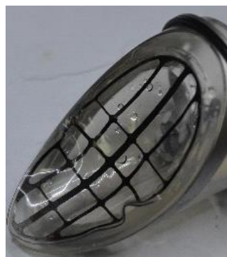
ZNP-Ti: flake deformation for: (1) dp = 100\text{mmHg} , (2) dp = 760\text{mmHg} , (3) after removal from the system. On the right: sealing of the valve under the deformation of the flap with pressure of > 400\text{mmHg} .
