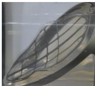
ZNP-S: (1) initial geometry, (2) deformation for dp = 300\text{mmHg} , (3) ditch is dp = 0\text{mmHg} . On the right: comparison of backflow of valves with a titanium and steel frame
