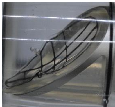
ZNP-Ti: flake deformation for: (1) dp = 100\text{mmHg} , (2) dp = 760\text{mmHg} , (3) after removal from the system. On the right: sealing of the valve under the deformation of the flap with pressure of > 400\text{mmHg} .
