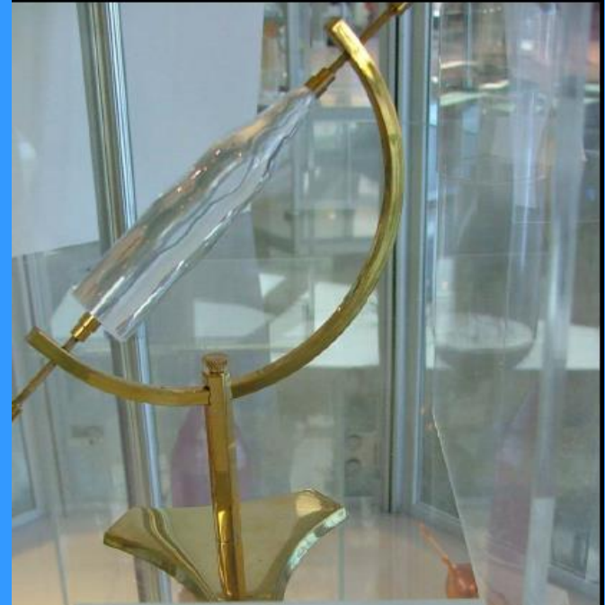
Al 2 O 3 PURE SAPPHIRE (CZOCHELSKI GROWN) courtesy of OAK RIDGE NATIONAL LABORATORY
