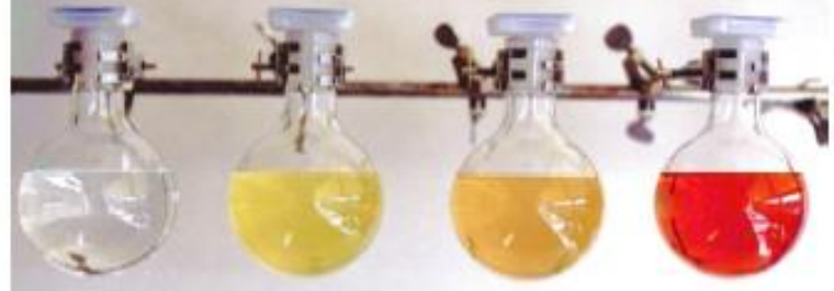
CdSe nano-particles in solution (1.5 - 4.0 nm)
