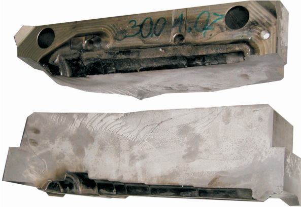
Fig. 1. Damaged die made of 50CrMoV18-30-6 steel
