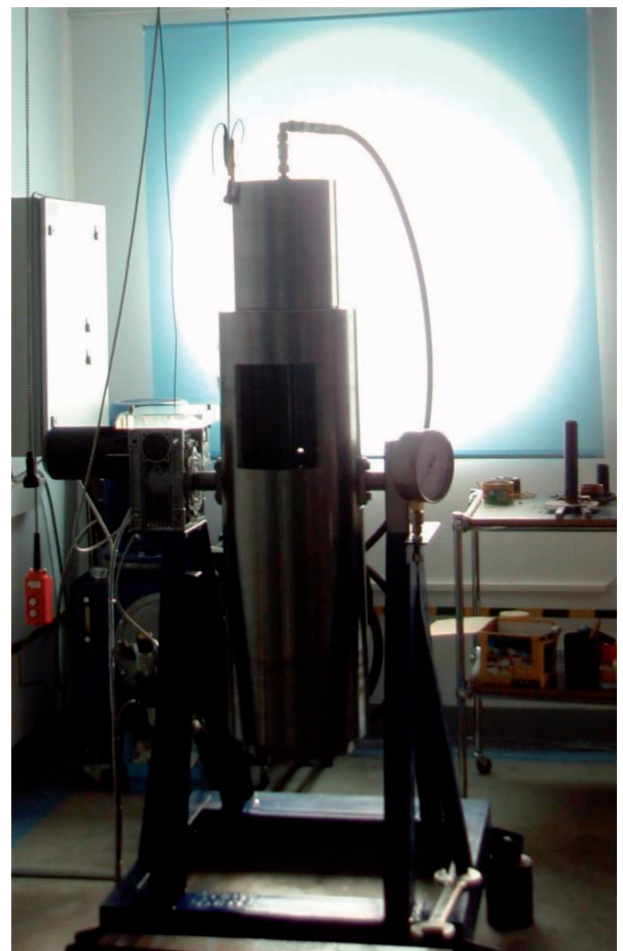
Fig. 3. Press for cold hydrostatic extrusion under a pressure up to 2.5GPa (designed and constructed at Unipress)
