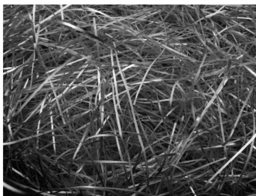
Fig. 7. The appearance of RS ribbon cast from AZ91 alloy
