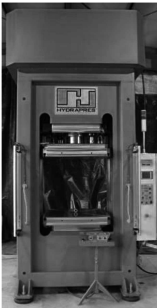
Fig. 5. Hydraulic press, max force 250T
