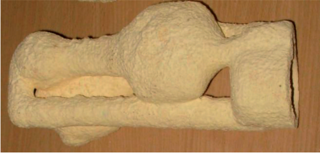
Fig. 7. Layered ceramic mould reproducing two connecting rods for an I.C. engine
