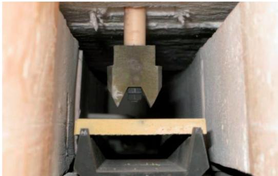
Fig. 4. The four-point strength measurement
