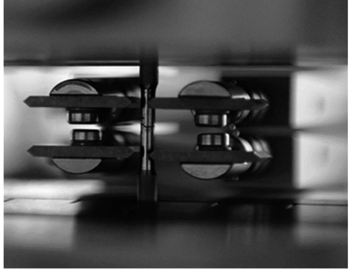
Fig. 1. A sample in a tensile strength tester with extensometer arms installed
