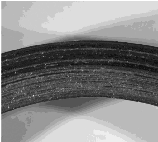
Fig. 8. Surface appearance of the ductile iron samples after the wear test
