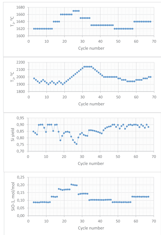
Fig. 2. Effects of the temperatures T_1, T_2 , on the Si yield in the Reactor 2 and the proportion of SiO(g) in the gas living Reactor 1 at equilibrium condition
