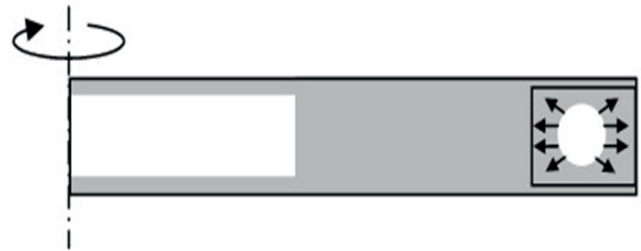
Fig. 6. Stage III – bubble compression inside preform; ← indicates the direction of capillary pressure
