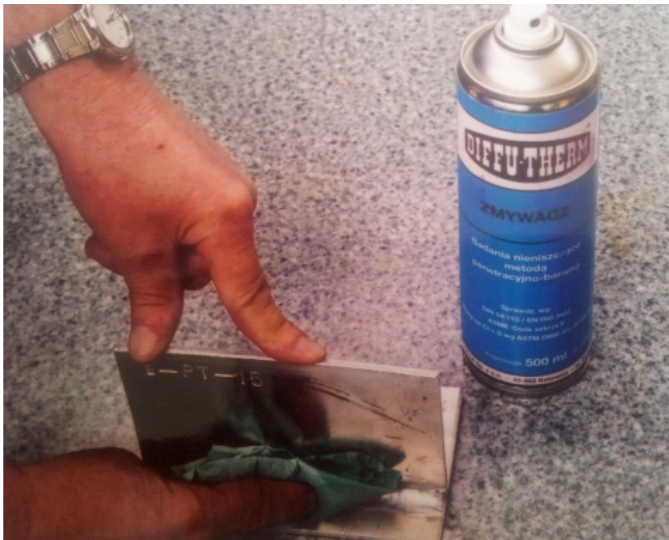
Fig. 3. Container with „Diffu – Therm” remover used for the removal of the excess of penetrant from the surface of the test fillet weld
