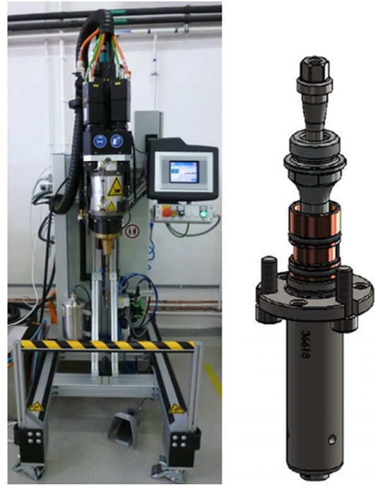
Fig. 1. RPS100 welding machine (left) and RFSSW tool (right)
