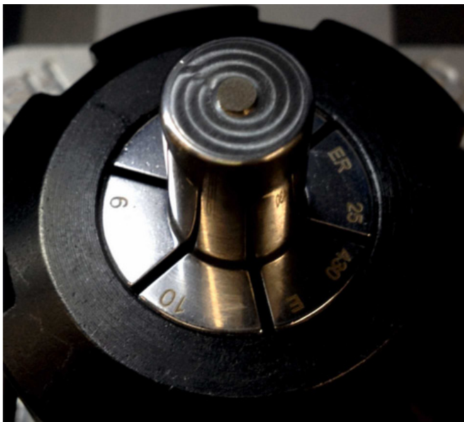
Fig. 4. The tool used in Friction Stir Welding process made from tungsten carbide
