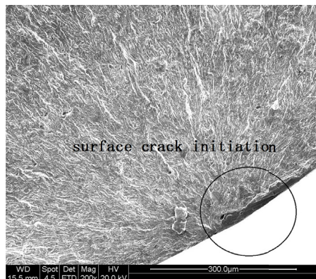
(a) Single crack initiation ( N_f = 1.76 \times 10^6 )
