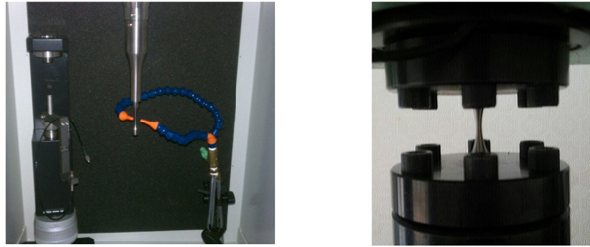
(a) The ultrasonic fatigue test system
