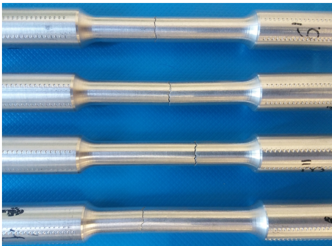
Fig. 10. Samples after a tensile test
