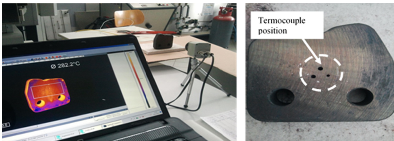
Fig. 1. Setup for the measurement (left) and the laboratory sample with indication on the position of the thermocouple (right)
