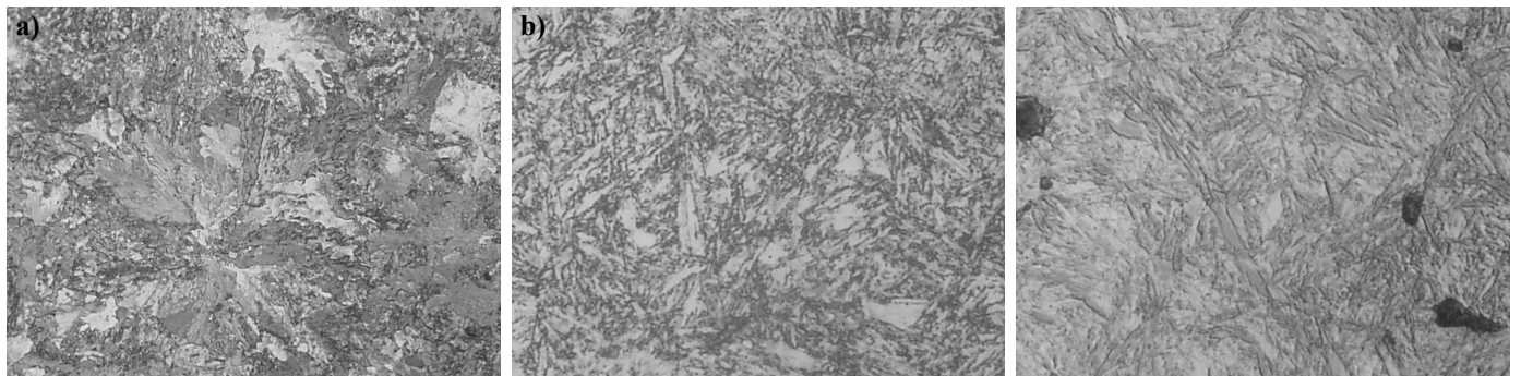
Fig. 4. Steel microstructure – zoom \times 1000 , cool. rate 30, 100 and 300 K/s
