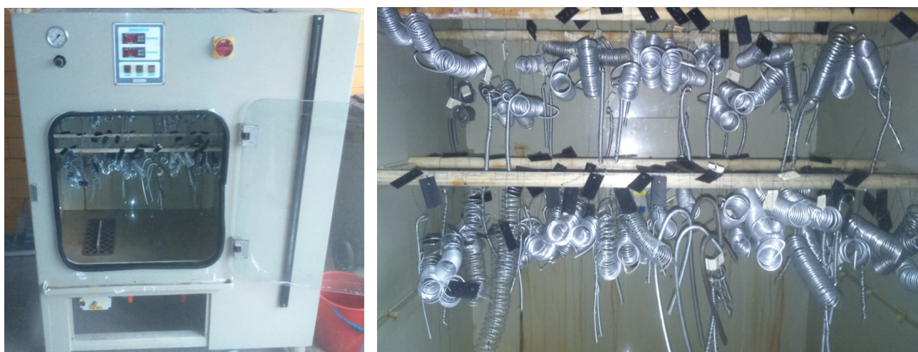
Fig. 5. The CORROTHERM Model 610 salt spray chamber
