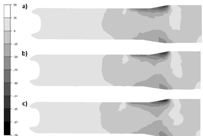
Fig. 4. Distribution of stress component \tau_{\rho z} during the rolling of the 20 mm magnesium alloy AZ31 round bar in three-high skew rolling mill: a) Variant I, b) Variant II, c) Variant III
