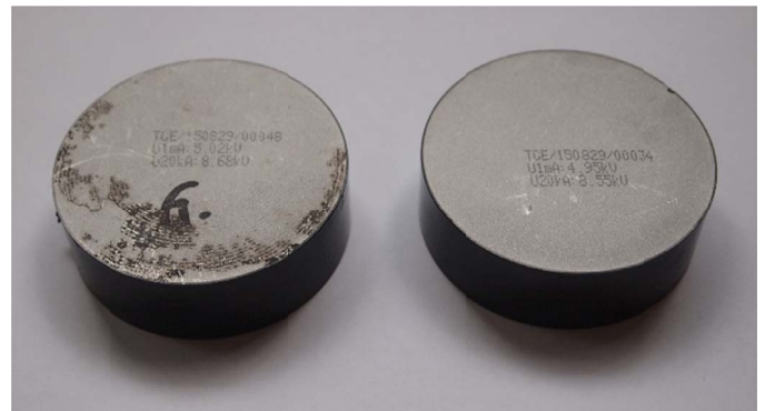
Fig. 2. Second pair of samples – varistor from a damaged 110 kV surge arrester on the left and an analogous – reference varistor that was not used
