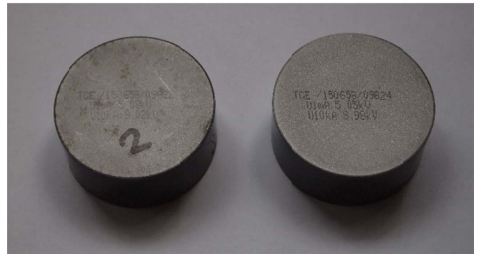
Fig. 1. First pair of samples – varistor from a surge arrester counter on the left and an analogous – reference varistor that was not used
