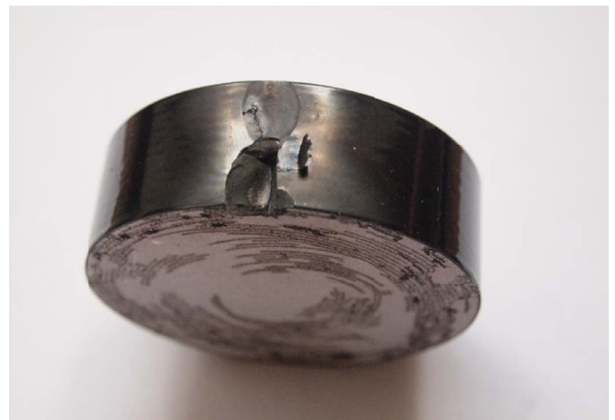
Fig. 3. Varistor from a surge arrester after a failure, with a well visible loss in the protective layer which resulted from strong short-circuit current flow
