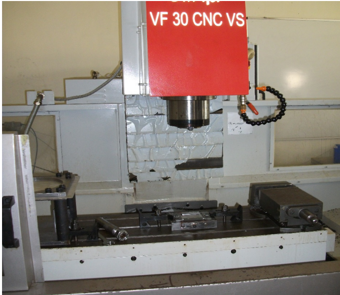
Fig. 1. Actual set-up on CNC vertical milling machine
