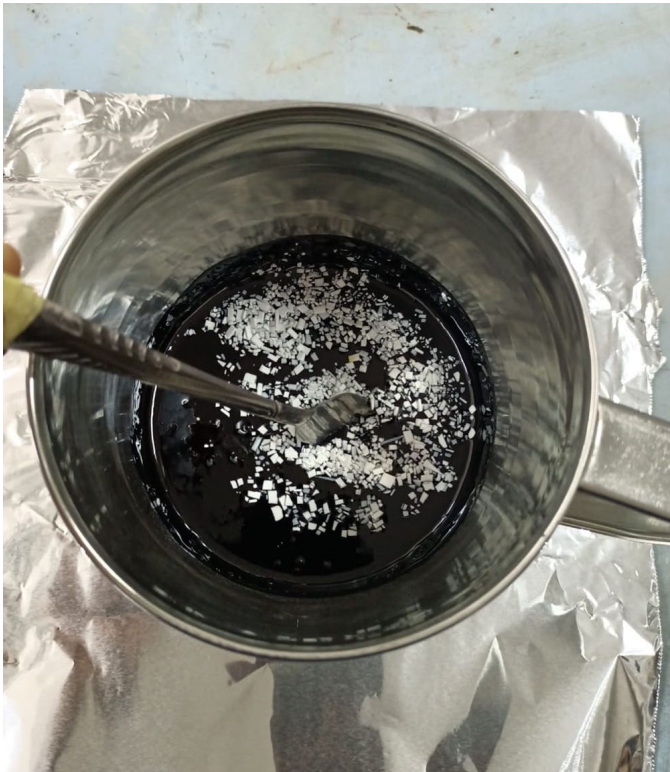
Fig. 1. HDPE plastic waste added into melted asphalt binder (Wet Process)
