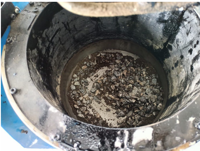
Fig. 2. HDPE plastic waste added into porous asphalt sample mixture (Dry Process)
