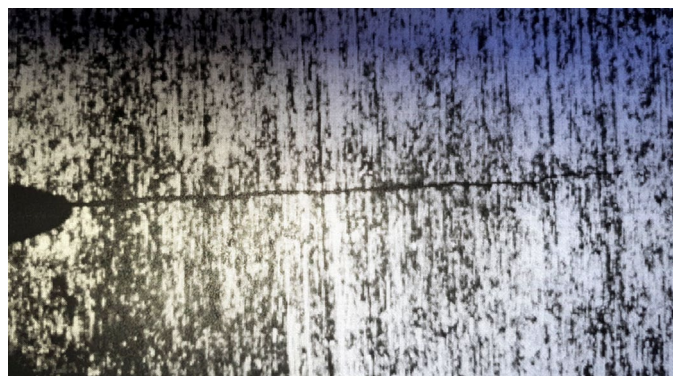
Fig. 2. Optical crack profile in LAMC225 MMC material at 225 MPa ( \times 100 ). 1.8 mm total crack length. Crack propagated from left to right
