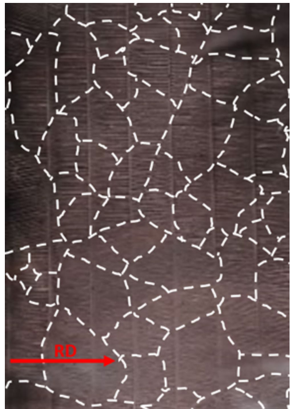
Fig. 7. Comparison of grain boundaries and domain boundaries by magnetic viewer method – sample No. 1
