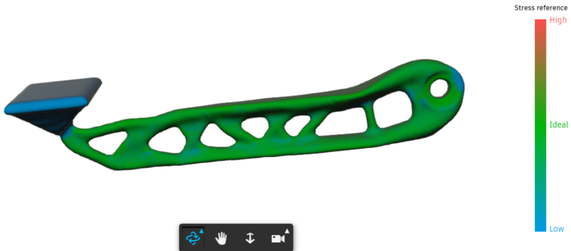
Fig. 13. Von Mises stress acting on the body
