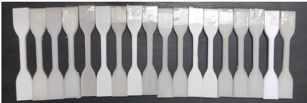
Fig. 5. (ASTM D638-14) 18 3D printed Tensile Strength test specimen
