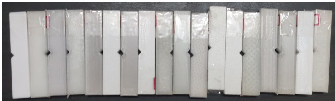
Fig. 4. (ASTM D256) 18 3D printed Izod Impact test 3D printed specimen
