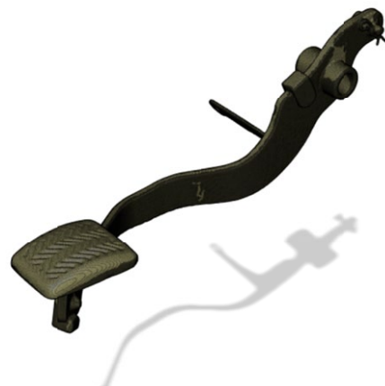
Fig. 1. 3D scanned model of the brake pedal
