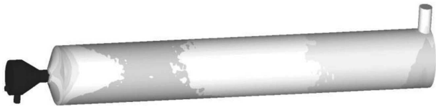
Fig. 5. View of the model with temperatures distributed at the walls of the chamber
