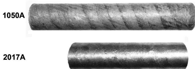
Fig. 9. Samples taken from the aluminum bars rolled in three-high skew rolling mill
