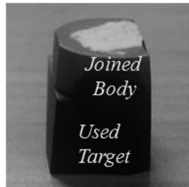
Fig. 4. ITO green body joined with used target by sintering at 1300°C for 2 h under 0.296 MPa
