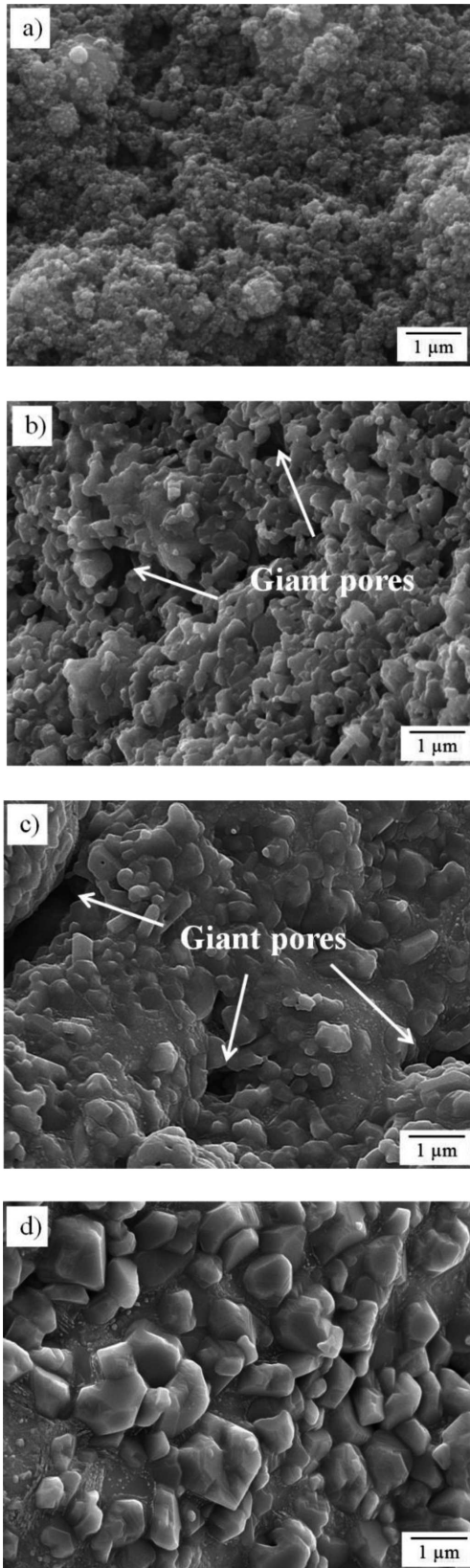
Fig. 6. SEM microstructures of sintered porous Fe-Cr-Al alloys; a) as coated and sintered at b) 1350°C, c) 1400°C and d) 1450°C for 2h
