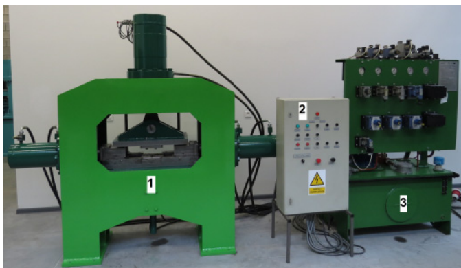
Fig. 4. Three-slide forging press: 1 – mechanical part of the press, 2 – control cabinet, 3 – hydraulic power system
