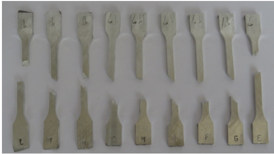
Fig. 14. Test specimens after fracture
