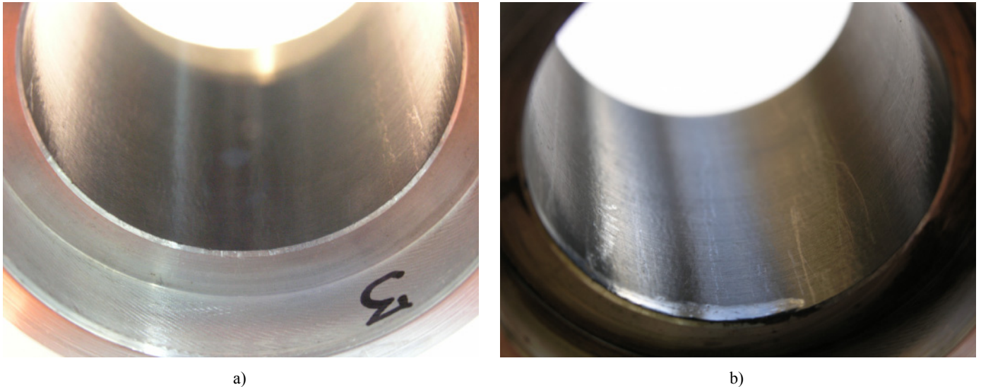
Fig. 8. Cylinder for oil less compressor before coating (a) and after coating with AHC+GC composite layer
