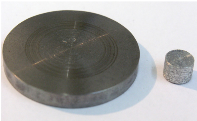
Fig. 6. Composite sample (pin) and countersample (disc) used for tribological investigation
