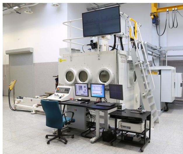
Fig. 1. The electron beam machine for welding and surface modification model XW150:30/756
