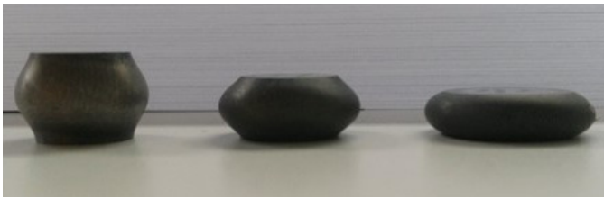
Fig. 1. Appearance of specimens after compression of 30%, 50% and 65%
