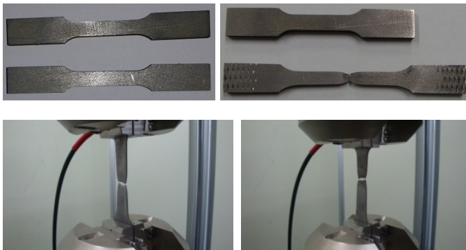
Fig. 2. Specimen tensile test
