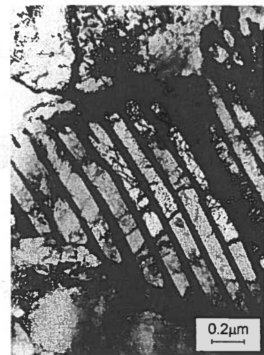
Fig. 7. TEM microstructure of the steel deformed with \epsilon_t = 0.3 during phase transformation at cooling rate of 2 K/s and strain rate of 0.004 \text{ s}^{-1}
