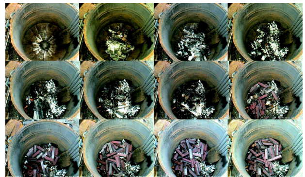
Fig. 3. Beginning of a scrap loading sequence for one basket
