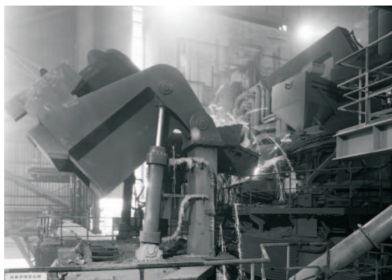
Fig. 2. Pouring of hot metal through EBT runner
