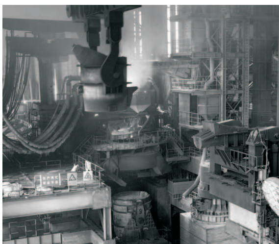
Fig. 3. EAF ready for tapping – exchange of hot metal ladle
