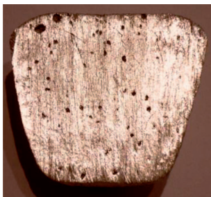
Fig. 1. Gas pores visible in Al-20 Zn alloy
