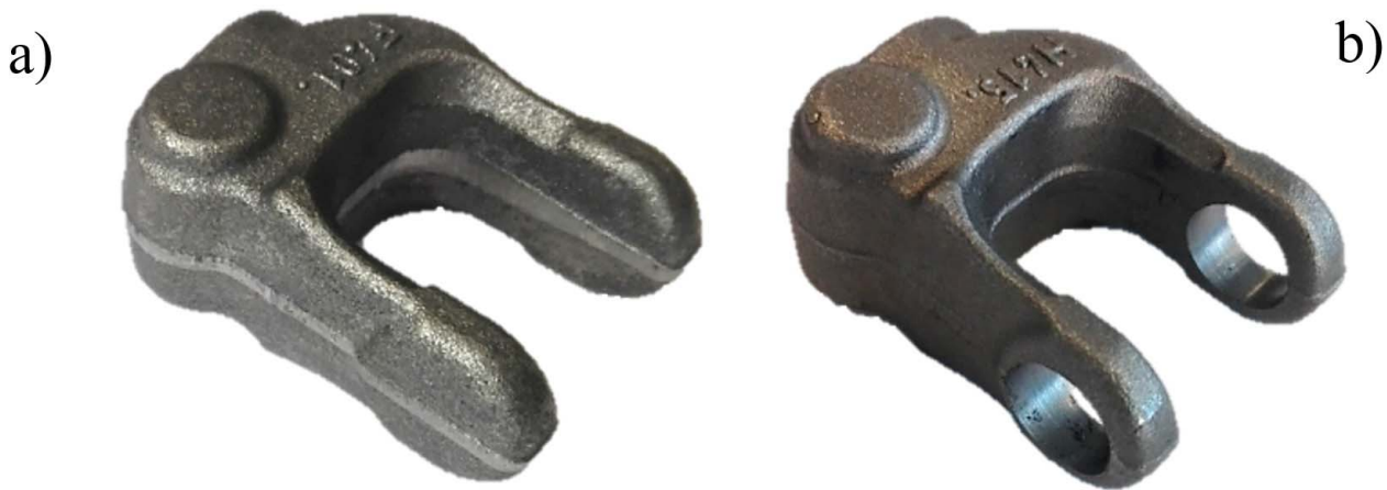
Fig. 11. a) final forging, b) sample prepared for the test
