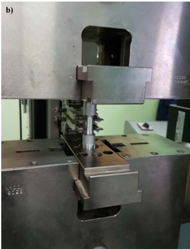
Fig. 3. ZWICK/ROELL Z100 testing machine (a) and the sample's mount (b)
