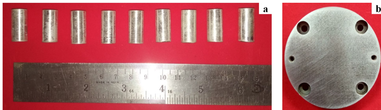
Fig. 1. (a) Wear pin samples, and (b) counterpart disc made of EN31 steel
