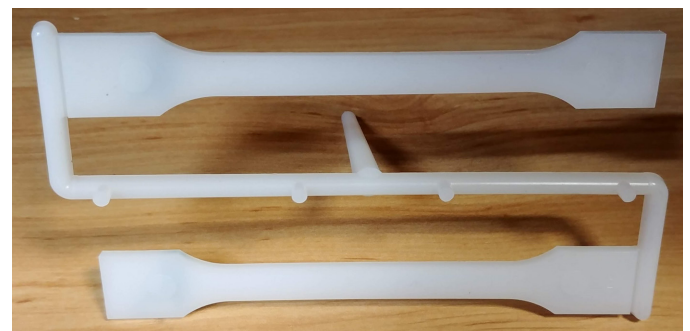
Fig. 3. The view of obtained molded part
