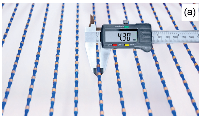
Fig. 3. The thinnest commercial diamond wire (a) and presentation of Premia MDW machine (b) at Marmomac 2017 held in Verona, Italy (Courtesy of Q-TEQ Ltd.)
